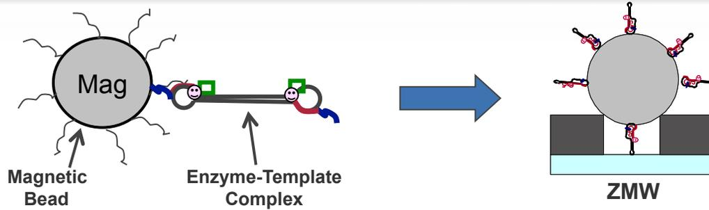
Multiple complexes attached to magnetic beads that are much larger than individual ZMWs
